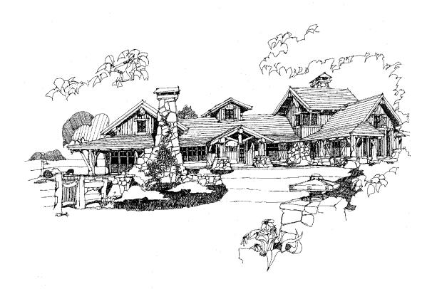
River Ranch McCall encourages form and massing that relate to the natural characteristics of the site. On sloping sites, the building form should step with the natural grade, and on level sites, the form should tend toward the horizontal. Massing should be higher at the center of the structure and lower at the outer edges. Designs with more floor area on the ground floor than on the upper floor will result in appropriate massing. Asymmetrical massing is encouraged
