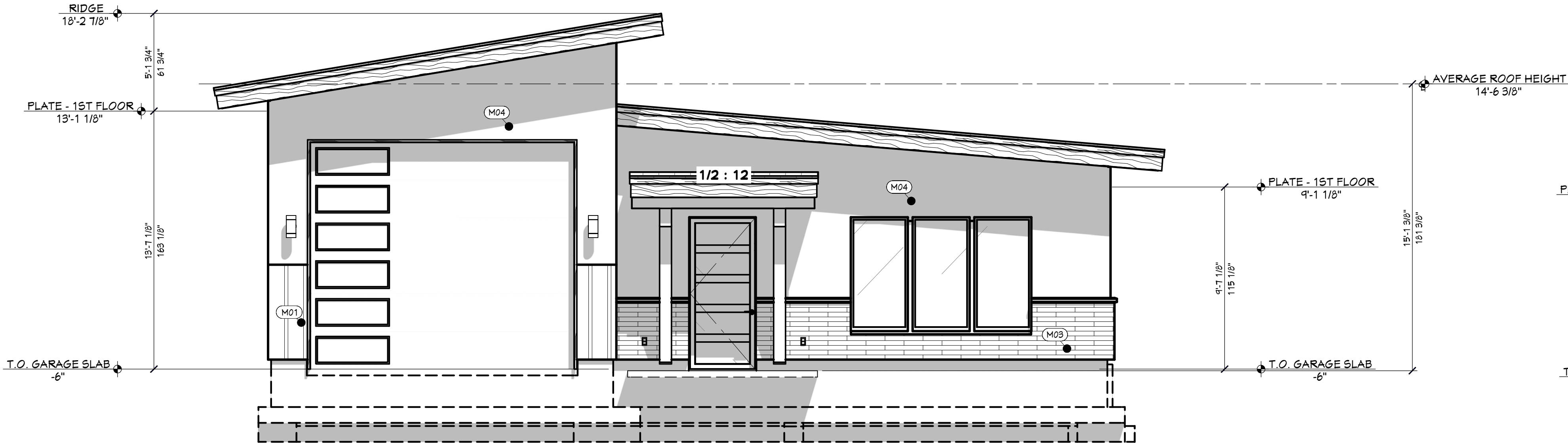
FT FRONT ELEVATION 1/4 IN = 1 FT
