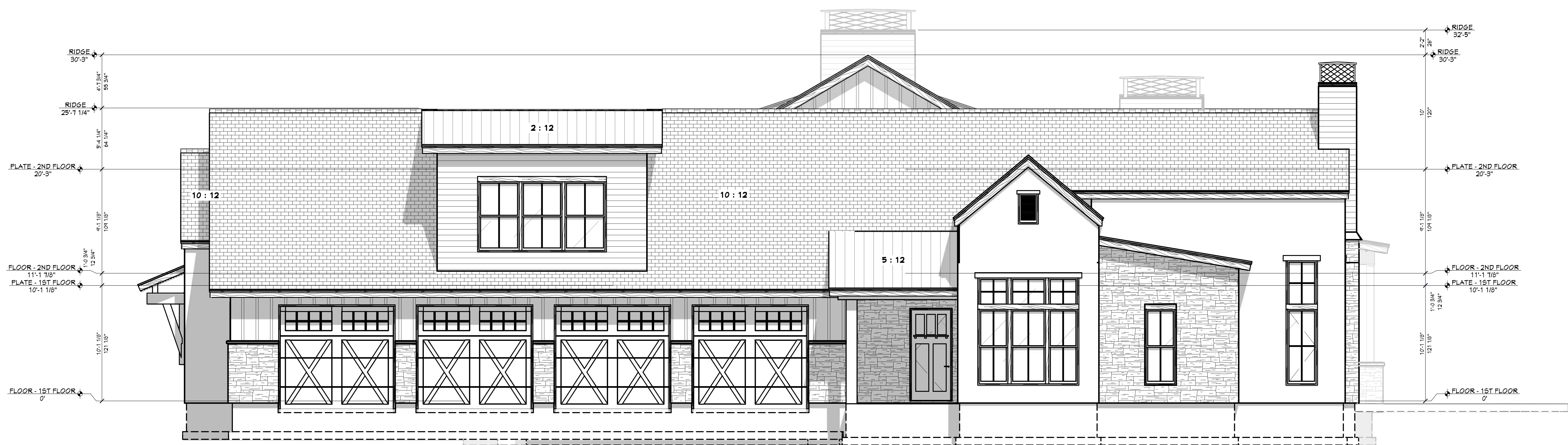
RT RIGHT ELEVATION 1/4 IN = 1 FT
