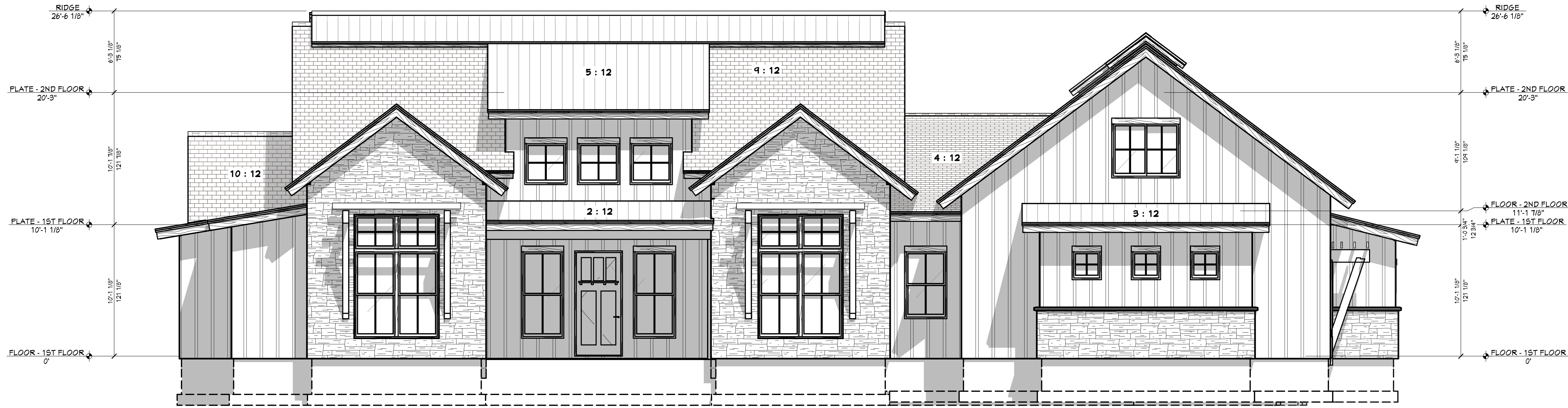
FT FRONT ELEVATION 1/4 IN = 1 FT
